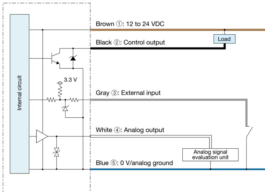
■ Analog output type: With the PNP setting
