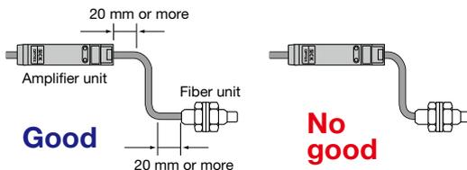
9. Because sensing distance may decrease by as much as 20% depending on the conditions of cut surface of the fiber or connection conditions with the amplifier, we recommend using with sensing distance set at 80% or below.
