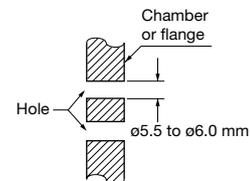
2. Mount the optical joint part to the vacuum chamber wall. When mounting to the vacuum chamber wall, the O-ring included with this product must be attached and the side to which it is attached must be the atmospheric side.
