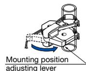
(Note 1): Sensitivity settings must be reconfigured after readjusting the mounting position.
