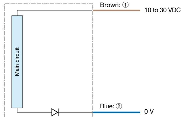
\*For the universal voltage type, add 24 to 240 VAC / VDC to the brown wire and blue wire. (No polarity)
