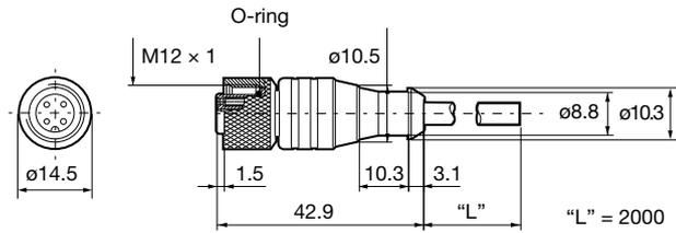
Cable section material: PVC, Conductor cross-section: 4-wire x 0.25 mm<sup>2</sup>
